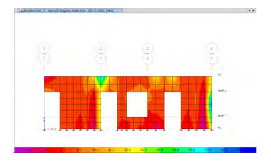
Out of plane Stress Analysis (Horizontal Direction)
