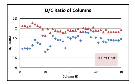
Figure 21: Demand Capacity Ratio of Structural Member (Column)
