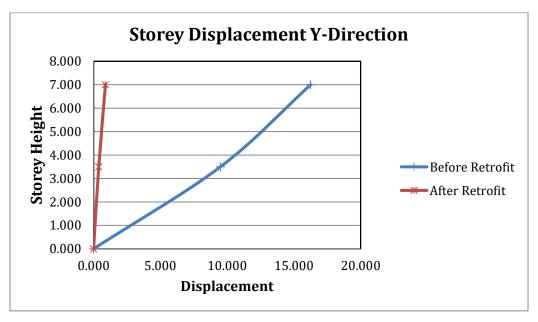
Figure 23: Storey Displacement Comparison
