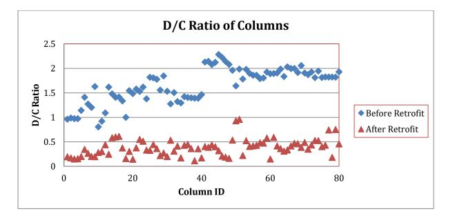
Figure 24: Demand Capacity Ratio of Structural Member (Column) after Retrofit
