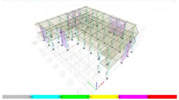
Figure 25: Demand Capacity Ratio of Structural Member (Column) after retrofit
