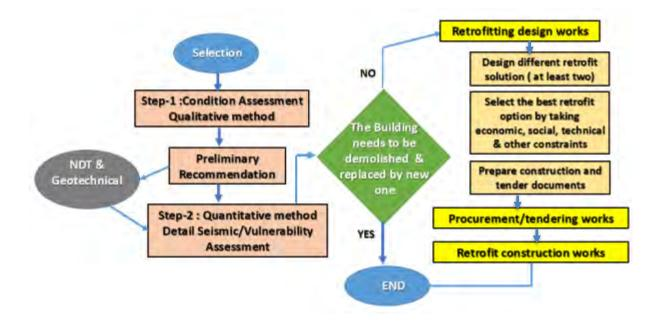
Figure 1: Flowchart of overall process of detail seismic assessment and retrofitting design
