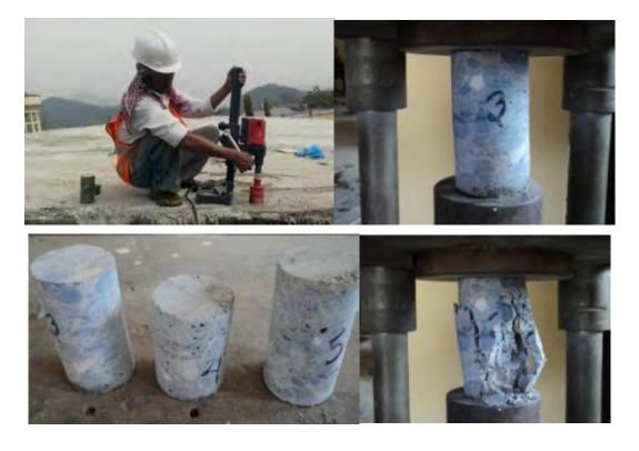
Figure 16: Photograph showing Concrete Core Test
