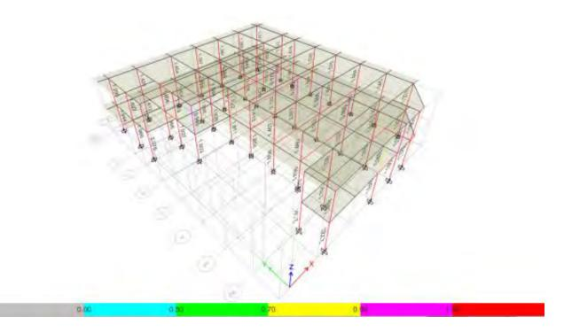
Figure 22: Demand Capacity Ratio of Structural Member (Column)
