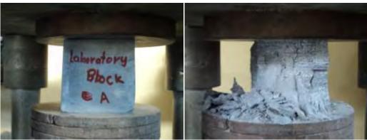
Figure 15: Photograph showing Compressive Strength Test of Stone
