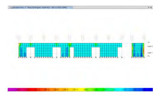
Out of plane Stress Analysis (Horizontal Direction)
