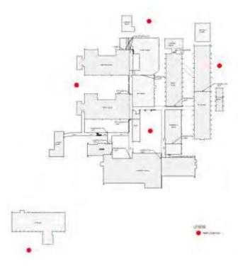
Figure 17: Location of Drill Holes for Geotechnical Investigation
