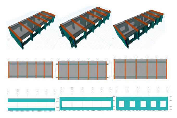
Case – I: Existing Building Case-II: Building with buttress & bands Case-III: Building with opening reduction
