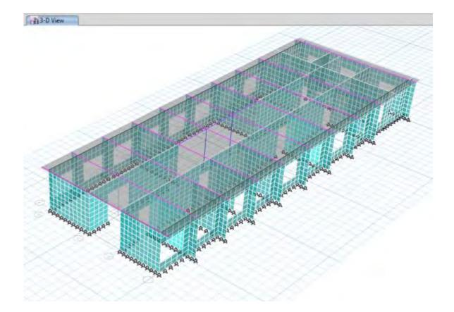
Figure 26: 3D Model of Building
