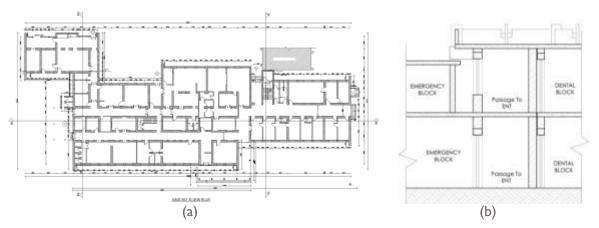
Figure II: a) Plan of Maternity Block. b) A disconnect load path in Emergency Block
