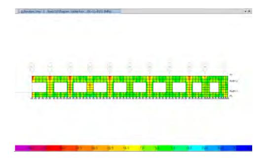
Out of plane Stress Analysis (Horizontal Direction)
